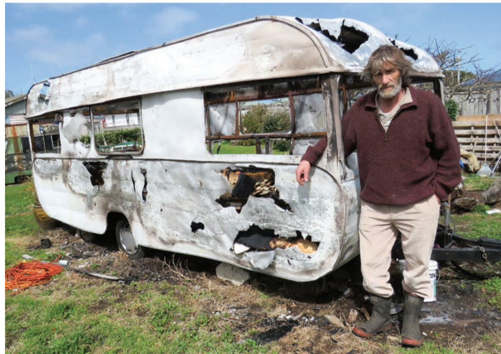
Graeme Powell and the remains of his caravan. Though the interior was plywood, the caravan was aluminium which also burnt and buckled in the fire.
